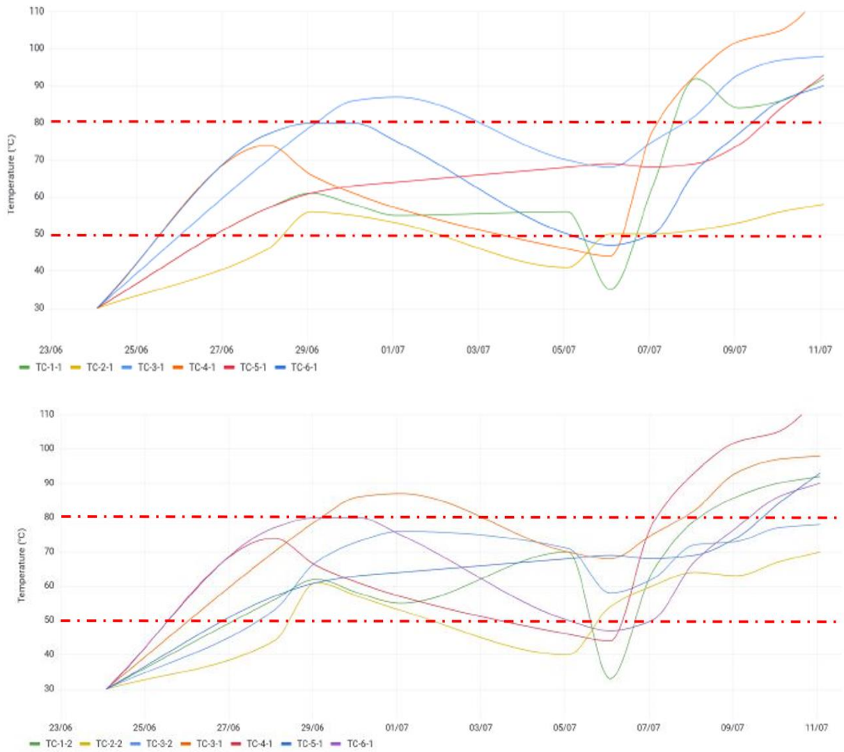
Figure 7. Soil temperatures during the in situ experiment in Heerlen (The Netherlands) were measured at the six measurement points at 1.5 m (top) and 3 m (bottom) depth. The temperature reached a plateau from the 29 th of June until the 4 th of July due to a fan malfunction. The two red lines represent the dual target temperature set at the beginning of the project.
