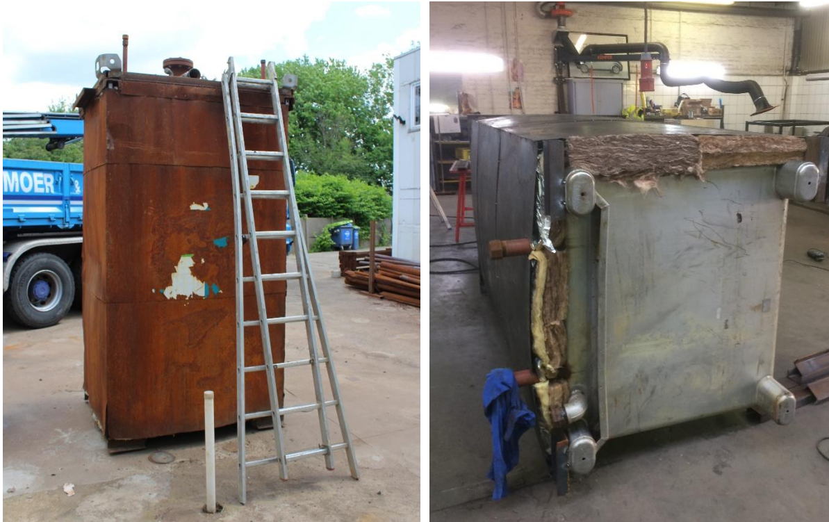
Figure 4. Left: The container for the ex situ experiment was filled with soil and Fallopia rhizomes. The soil in the container was heated through a steel pipe inserted in the middle of the container. Right: The container is insulated to minimize heat loss at the sides.
