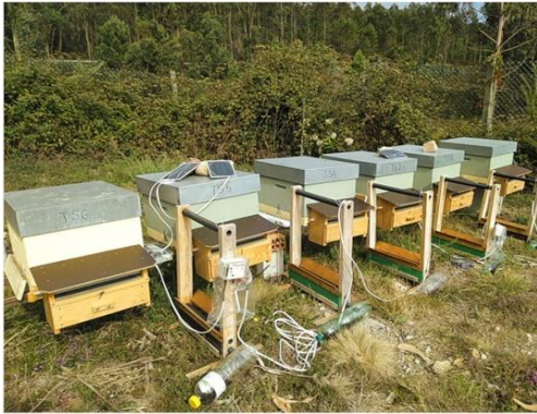
Figure 3: Set up of the electrical harps in front of the beehives, perpendicular on the flight direction of the bees (Rojas-Nossa et al., 2022).
