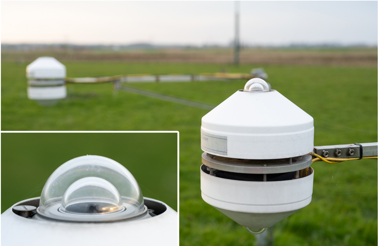
Figure 1.4: Thermopile pyranometers to measure solar irradiance. On the right are two thermopile pyranometers, one facing up and one facing down, which together measure net solar irradiance. The bottom left is a zoom in on the black surface beneath a glass dome that heats up in response to radiation. This one could use cleaning. Out of focus in the top left are two instruments to measure incoming and outgoing long wave radiation.
