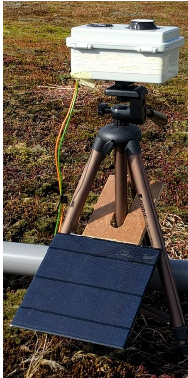
Figure 3.2: FROST with solar panel mounted on a camera tripod.
