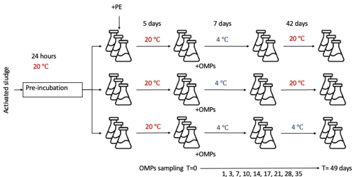
Fig. 1. Schematic representation of the biotic batch test.
