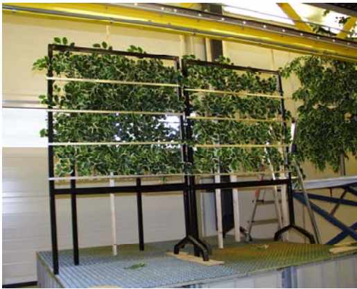
Fig. 2. Leaf walls (left) and artificial tree (right) as setup in the spray chamber alongside the spray track in the IMAG spray laboratory.
