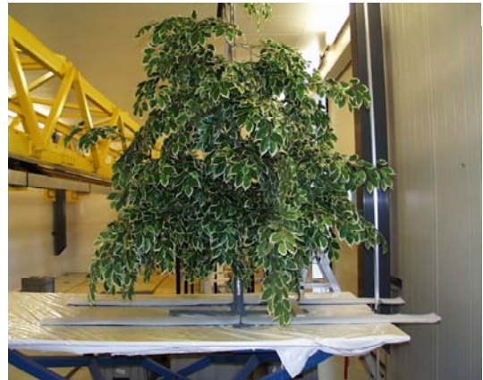
Fig. 2. Leaf walls (left) and artificial tree (right) as setup in the spray chamber alongside the spray track in the IMAG spray laboratory.
