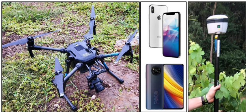
Fig. 6. Equipment Used in the Study. Left: DJI M210 Drone. Middle: Smartphones - iPhone X (top) and Xiaomi Poco X3 Pro (bottom). Right: Trimble R2 Integrated GNSS System.
