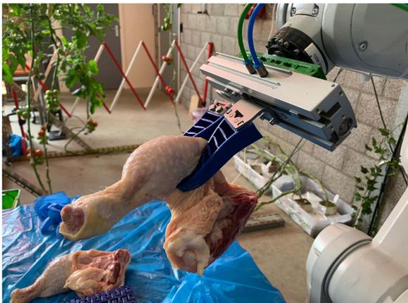
Fig. 10. Example picture of the Festo gripper that adapted to the shape of the chicken piece to firmly grasped it during the picking and placing operation in one of the experiments.
