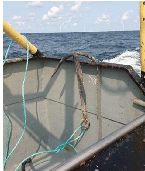
Figure A5.3: 29/08/2023 light dredge anchor used for recovery of string without markings
