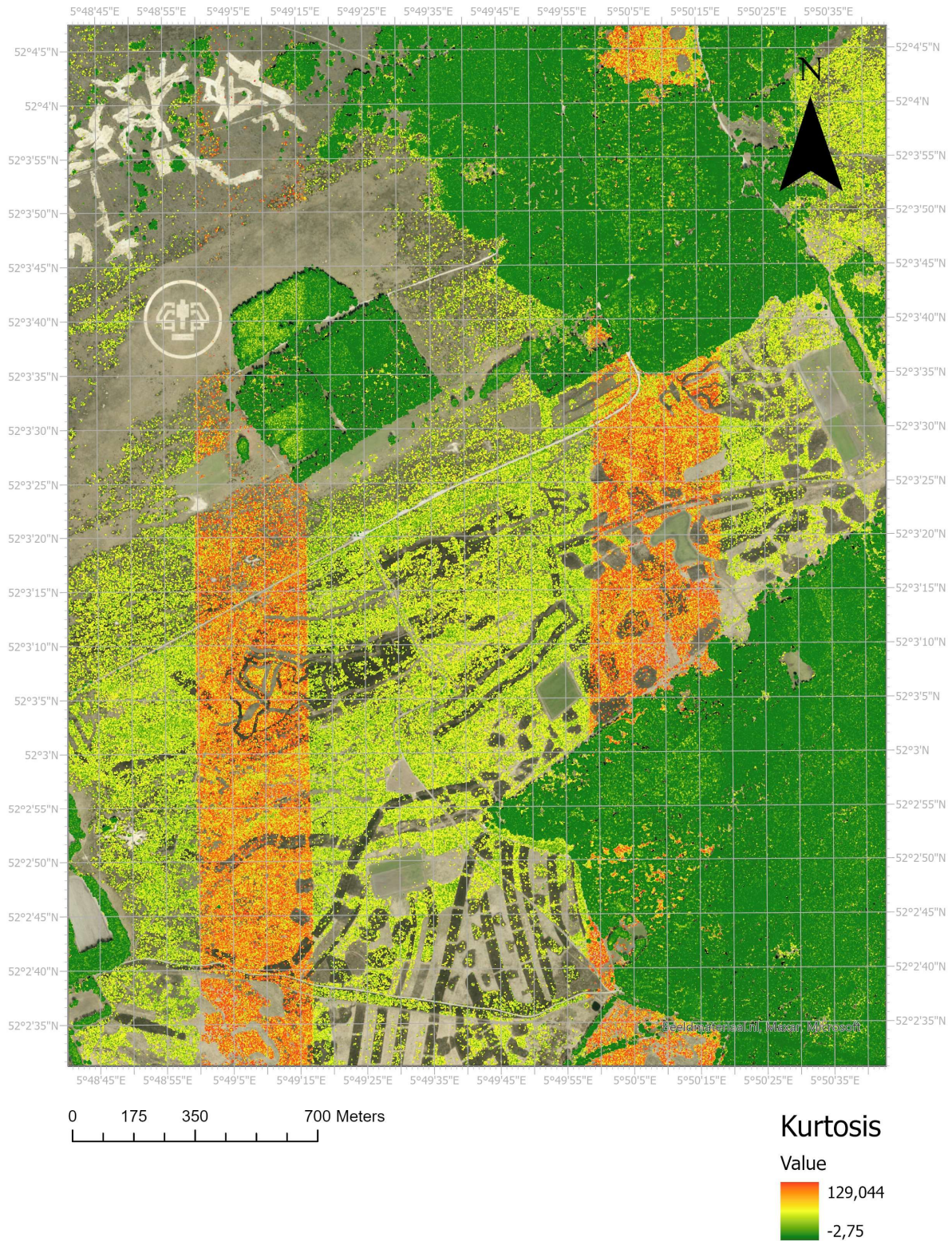
Figure 16: Layout showing higher kurtosis values at the locations where flight routes overlap. The orange stripes indicate these overlap areas.
