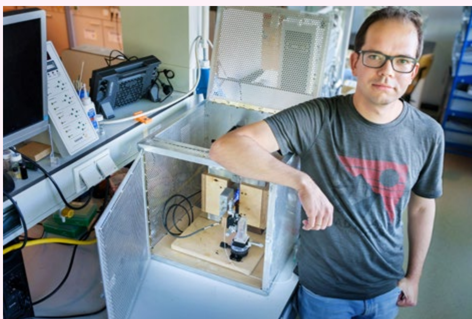
The NMR spectrometer stands in a metal cage in the lab to protect it from interfering FM radio waves. Researcher Sander Baas, the designer of the instrument, explains, 'The NMR radio pulses are at around 90 MHz, and FM radio broadcasts at 87-108 MHz. That's why we have this Faraday cage.' ♦ Photo Guy Ackermans
