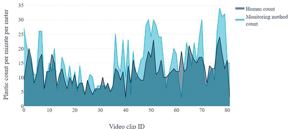
Figure 9. Performance of automatic feature detection for plastic detection applied on five different river locations across Jakarta, Indonesia (taken from van Lieshout et al. 2020).
