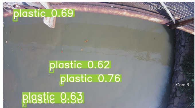
Figure 10. Sample image of floating plastic bottles in the environment, with floating macroplastic processed with the YOLOv7 algorithm.
