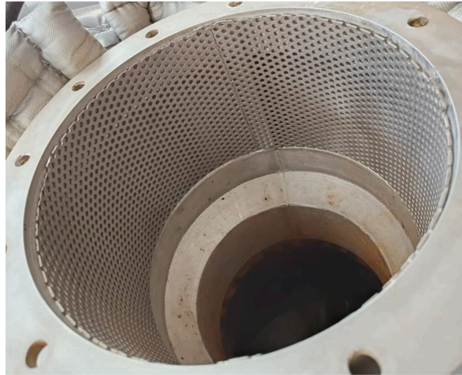
Fig. A1. Detailed picture from the perforated basket inserted in the air distributor.
