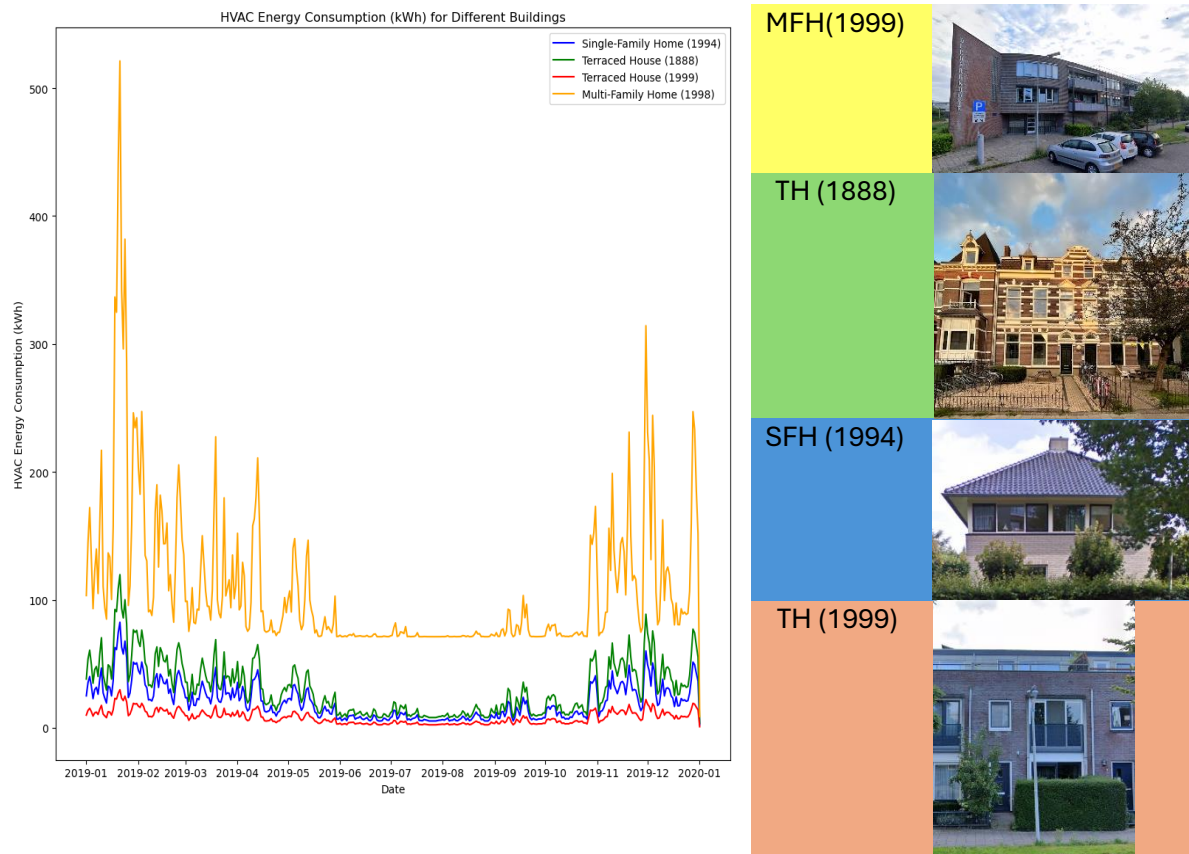
Figure 3.10 Graph of daily energy demand fluctuations for four sample buildings, each belonging to a distinct building class. (MFH = Multi-Family Home, TH = Terraced House. SFH = Single Family Home)
