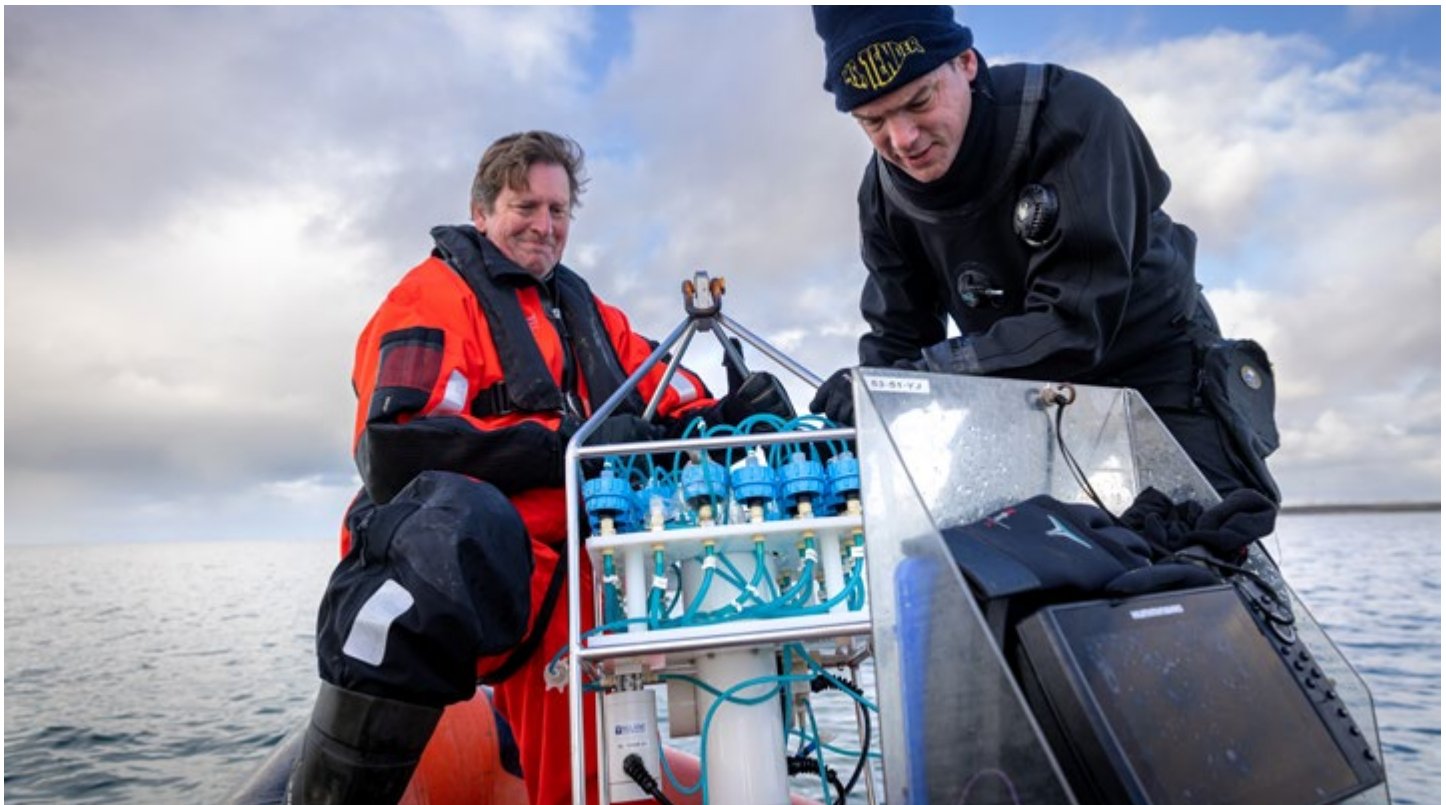
Marine biologist Reindert Nijland (right) and PhD candidate Niels Brevé with the sensor box on the Hinderplaat intertidal flats in Zuid-Holland. Nijland is developing the device to perform e-DNA measurements at sea • Photo Anne Reitsma
