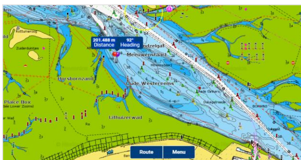
Figure 4-8. Depth profiles in part of Ems estuary (source: webapp.navionics.com ). The (small) bar indicates a width of 200 m, the approximate size of the gillnet.
