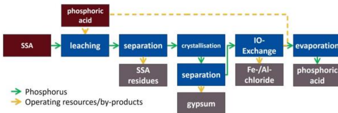
Figure 11 Phosphoric acid production scheme of TetraPhos® (Ploteau et al. , 2021b). P is extracted from SSA using P-acid. Thereafter, purification steps as filtration, crystallization by addition of sulphuric acid, ion exchange, and evaporation are used to produce P-acid.
