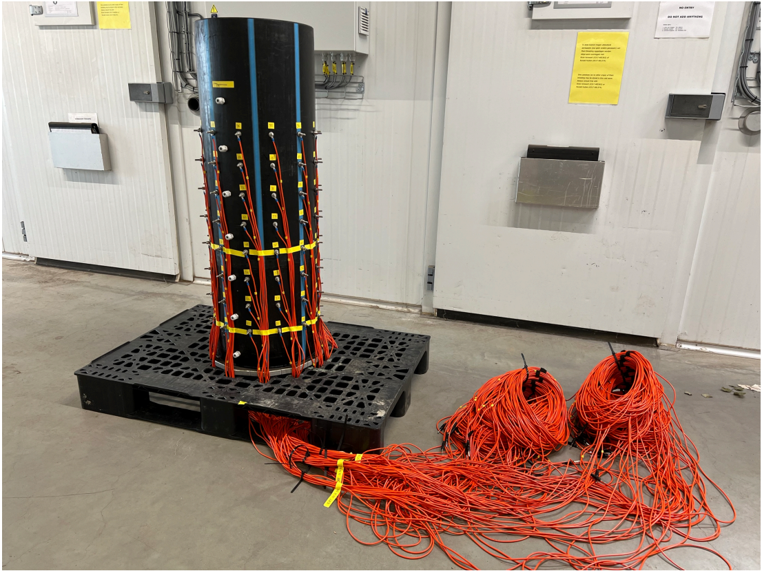
Figure C.2 | Photo of the column setup showing the HDPE column, electrodes located around the circumference, and orange wires connecting all of the 96 individual electrodes to the switch boxes, that connect to the Syscal ERT.
