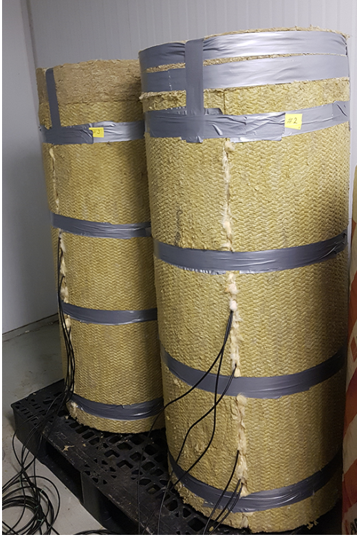
Figure 3.1 | Photo of two out of nine columns during the freeze/thaw experiment. Each column of 1.2 m high and 0.315 m diameter is wrapped in 0.12 m thick insulation material held in place with duct tape and placed on a plastic pallet to isolate it from the ground. Also visible are the temperature sensor cables that come out of the insulation.
