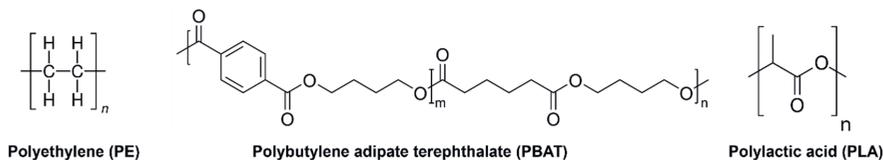
**Figure 1.3** Chemical structure of commonly used plastic polymers in agriculture: fossil-based polyethylene (PE), fossil-based polybutylene adipate terephthalate (PBAT) and biobased poly(lactic acid) (PLA)
