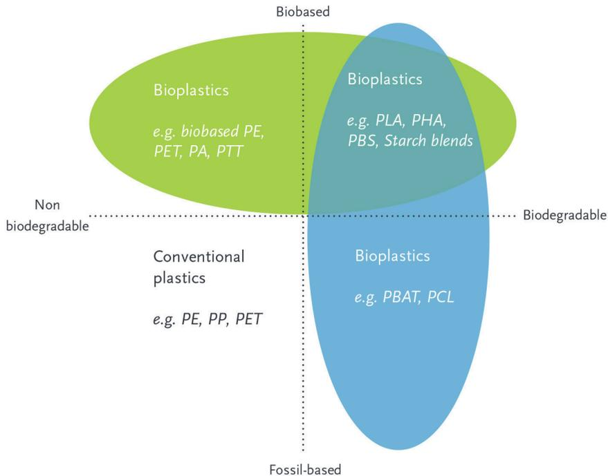
**Figure 1.2** The coordinate system of plastic materials. Source: Fact Sheet of European Bioplastics (2016).
