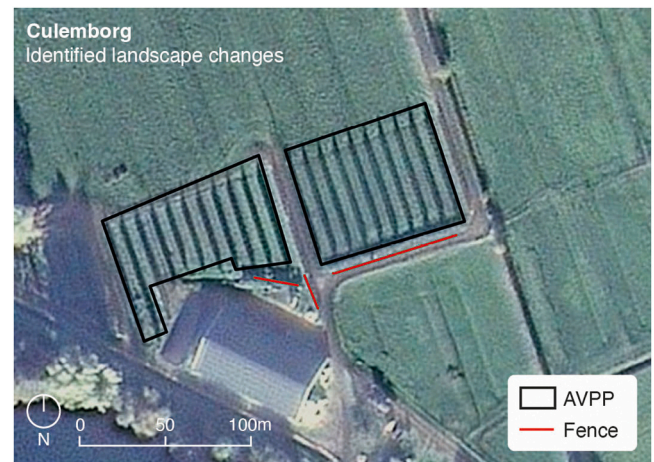
Fig. 6. Culemborg site with identified landscape changes. AVPP stands for agrivoltaic power plant. The basemap is a satellite image taken in 2023 (Satelietdataportal, 2023).
