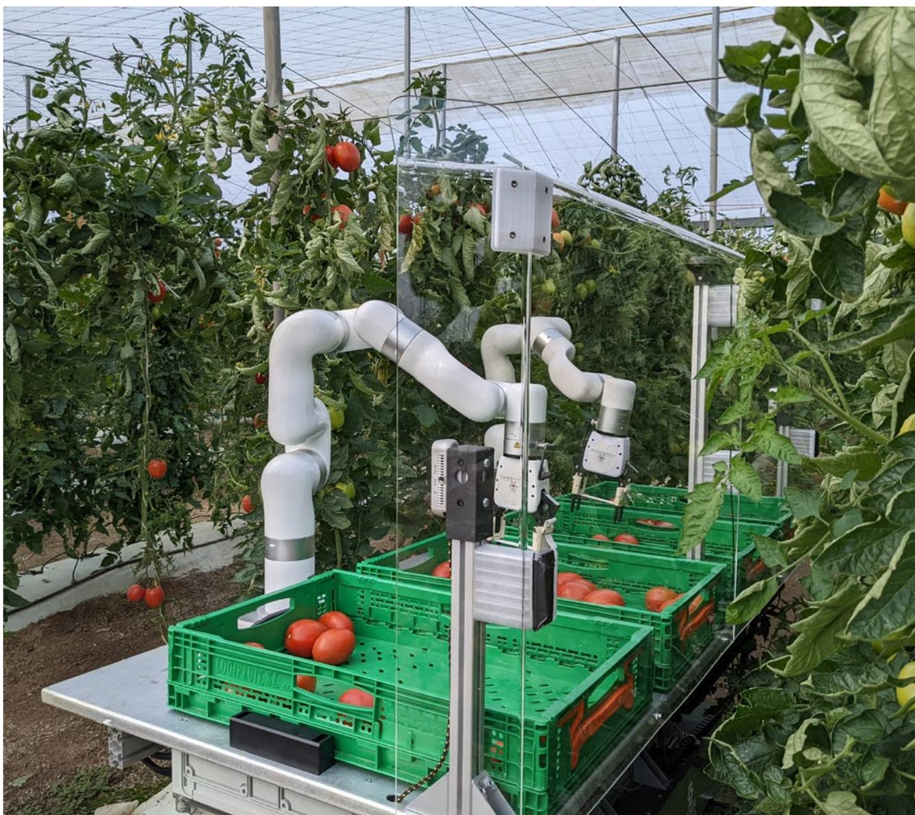
using the folding-over-wire method. This method results in a complex environment with variable tomato density and obstructions caused by leaves and wires. This type of environment makes both detection and harvesting much more complicated. Both detection and harvesting algorithms were adapted to the new environment and good results were achieved. However, results couldn't fulfil all expectations that would have been demonstrated by testing multi-tunnel-high-hanging tomatoes.
