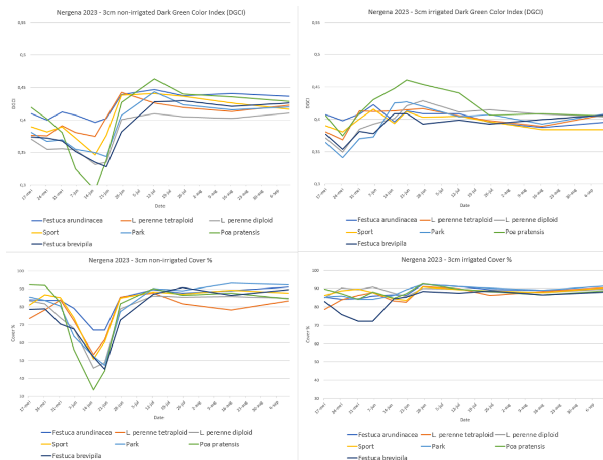
Figure 7.12: DGCI and Cover % 2023 3cm cutting height. On the y-axis, either Cover % or Dark Green Colour Index (DGCI) is displayed. On the x-axis, date of measurement is displayed. Measurements were performed once per week on average. Each line resembles a minimum of 3 plots and line colours are explained in the legend below the graph.
