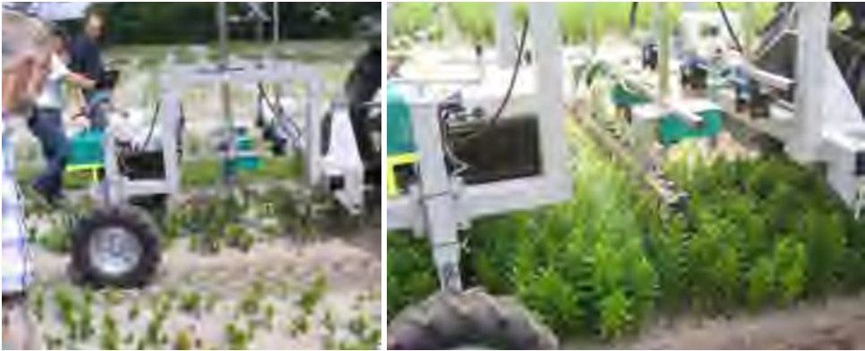
Figure 4. Prototype Canopy Density Sprayer for bed grown crops used in a lilly crop; left in early growth stage still individual plants; right in late growth stage with fully covered bed.
