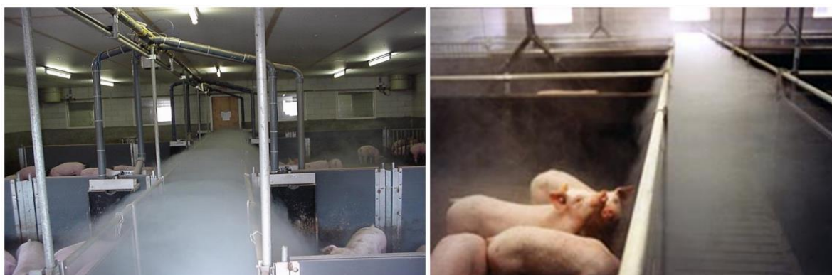
Figure 5.2.4: Examples of a smoke test with fresh air slowly entering the pig pens (©WUR)
