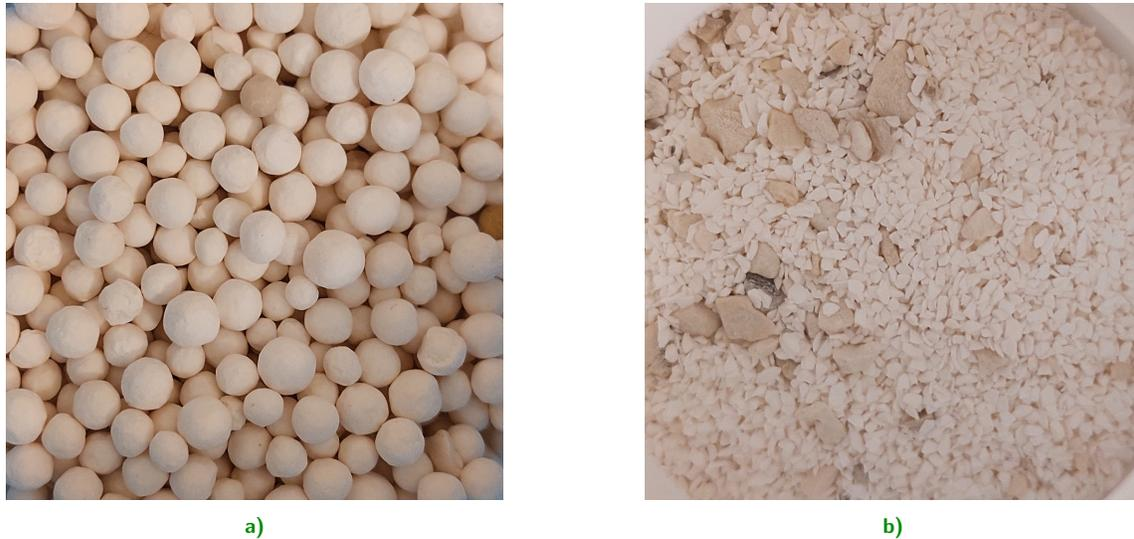
**Figure 1 – Two in-stream phosphate adsorbents** – The two products side by side. (a) shows Phosflow pellets™ and (b) shows EutroSORB® F. These pictures were taken by the author.
