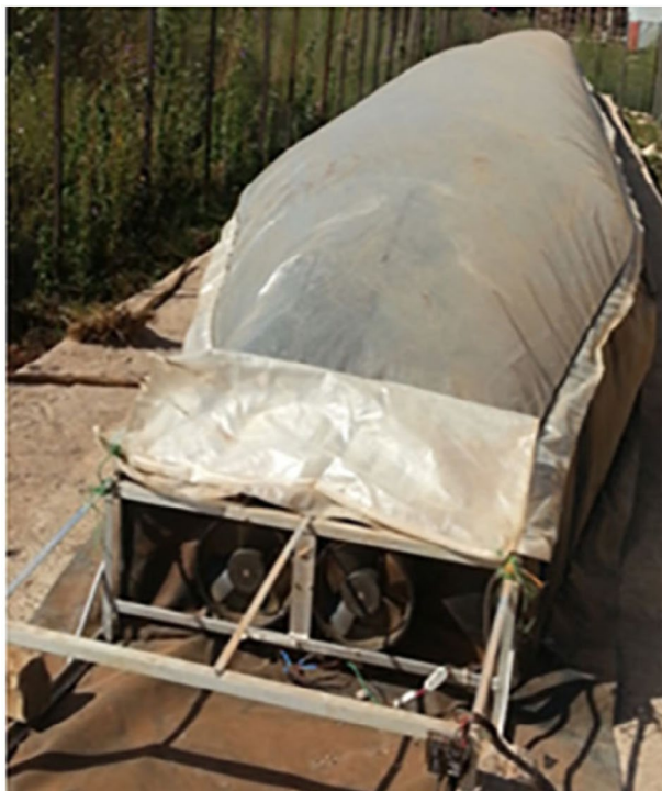
FIGURE 3 A solar bubble drier (photo with permission from GrainPro ® ; Asemu et al. , 2020).
