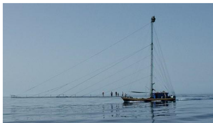
Figure 4: A “passerella”, shown with a typical “antenna” of between 15-25 m tall where a spotter stands. Once a swordfish is spotted, a harpooner will stand at the end of the ≈30-meter-long bridge that is mounted at the bow of the vessel, to strike the shot (Daniele Riefole, 2023; Palladino et al., 2019).
