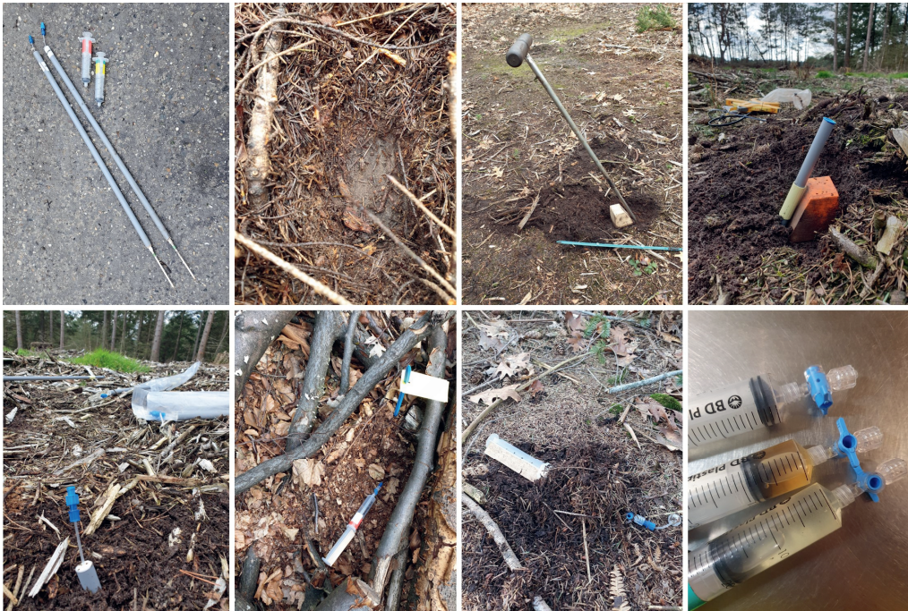
Figure 6.1 Overview of the macrorhizons used (top left) and the installation of the macrorhizons in the field. First, a small part of the organic layer was removed till the mineral soil (top middle left) and then the macrorhizon was placed under an angle of 30°, by using a gouge (ø15 mm) (top right). Soil moisture was sampled by attaching a syringe to the macrorhizon (bottom left), which was covered by organic matter in the field. Samples within each plot showed large heterogeneity as shown by three syringes which were taken from a stem only harvest plot in a clearcut (bottom right).
