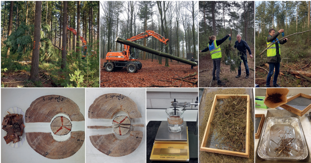
Figure 4.2 Pictures of measurements in the field (top) and in the laboratory (bottom). Fieldwork included measurement of the fresh weight of the entire tree (top left), fresh weight of the stem (top middle left), fresh weight of branches (top middle right) and fresh weight of the coarse branch (top left). Laboratory work included separation of the stem disk into bark, sapwood and, if present, heartwood (bottom left), extracting slices for determination of volume (bottom middle) and separation of the dried branch material into needles (bottom middle right) and small branches (bottom right).
