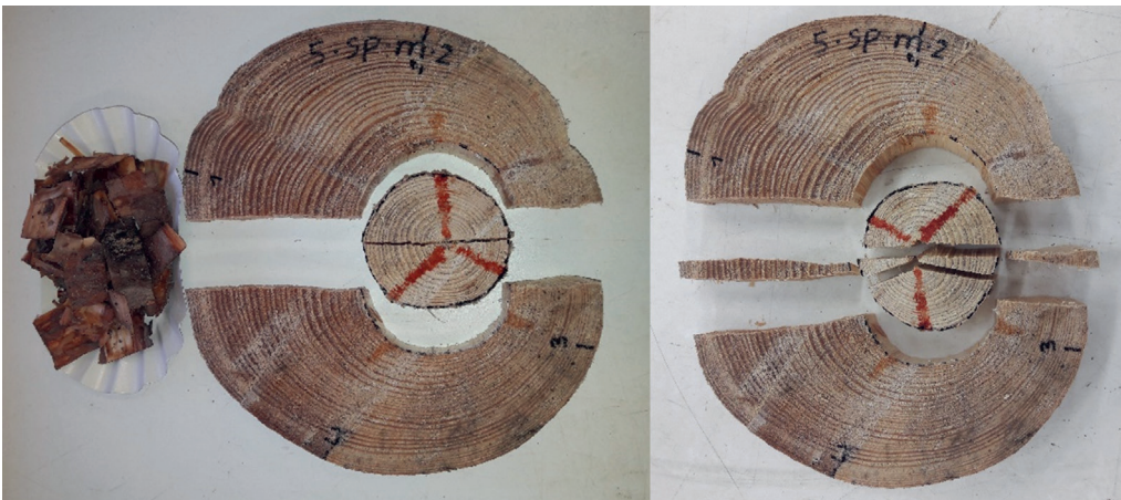
Figure S4.2 Separation of the bark, sapwood and heartwood (left) and the extraction of sapwood and heartwood pieces for the fresh weight to dry weight conversion and the density measurements.
