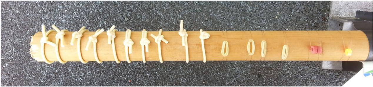
**Figure 1.** Experimental set-up to test deterioration rates of harness material. From left to right: 10 samples of harness material, four samples of latex ring material, one sample of a rubber ring and one sample of a PVC ring. In total four of these wooden sticks were placed under different conditions: in the sun, in the shade, in saltwater and sun, and in complete darkness.
