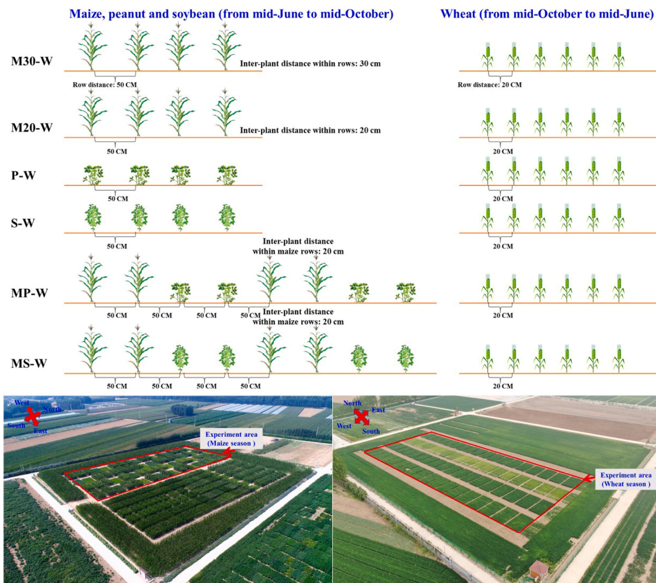
Fig. 1. Schematic diagram of six different double cropping systems with wheat (W) as a winter crop and maize (M), peanut (P), soybean (S), maize/peanut intercropping (MP), or maize/soybean intercropping (MS) during summer, and aerial photograph of the experiment area during the maize and legume growing season in summer 2019 and during the wheat growing season in the spring of 2021. Note that the photos made during the spring and summer seasons were made from a different direction (see direction markers).
