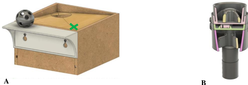
A B Figure 1 (from Marcus Clauss). The enrichment device, created by Marcus Clauss. It consisted of two components; the ball receptacle (A) and food dispenser (B) that were connected by a Raspberry Pi. A) Ball receptacle with the ball on the platform. The platform was not used in this experiment, so the ball was located on the green X mark in the figure at the beginning of each trial. The food dispenser had a declining slope, so the ball would roll in on itself when nudged. B) Food dispenser, made of plastic and created by a 3D printer. It has two levels that rotate (when activated by ball delivery) so kibble would fall out, and to ensure the same amount of food every turn.
