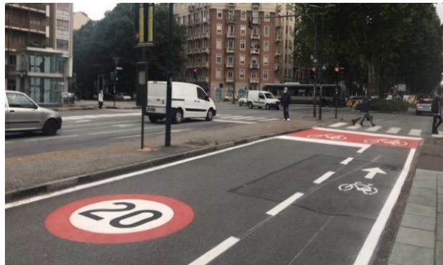
Figure 3. 'Controviali' in Turin with bike-priority and 'case avanzate' in front of each traffic light (Parisotto, 2020).
