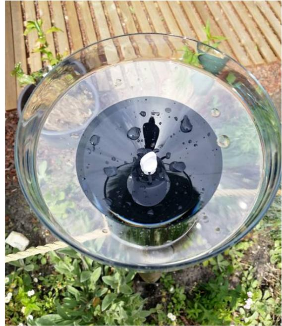
Figure 2.1: Topview of a Netatmo rain gauge module. Source: <http://www.at-smartliving.com/netatmo-rain-gauge-clouds-pass-but-rain-remains/>. (Published: May 21, 2019).
