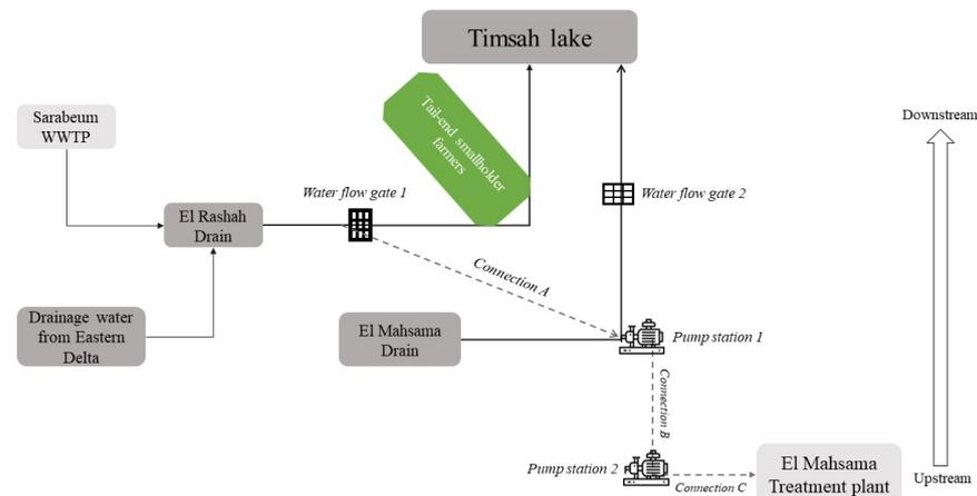
**Figure 4.** Water flow diagram in the study area of Al Mahsama.
