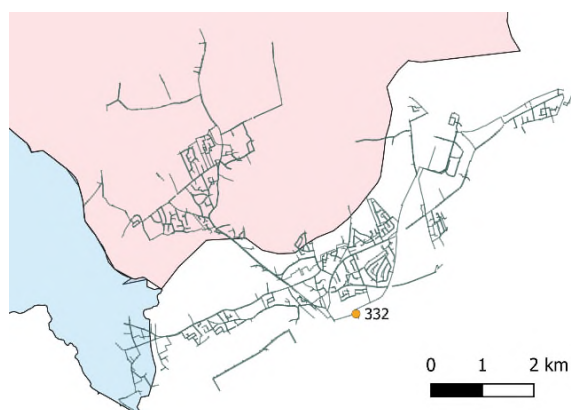
Figure 73: The orange dot shows the location of the available observation from the MOS dataset and its ID. The grey lines gives the sewage system as represented in 'State A' from InfoWorks CS.
