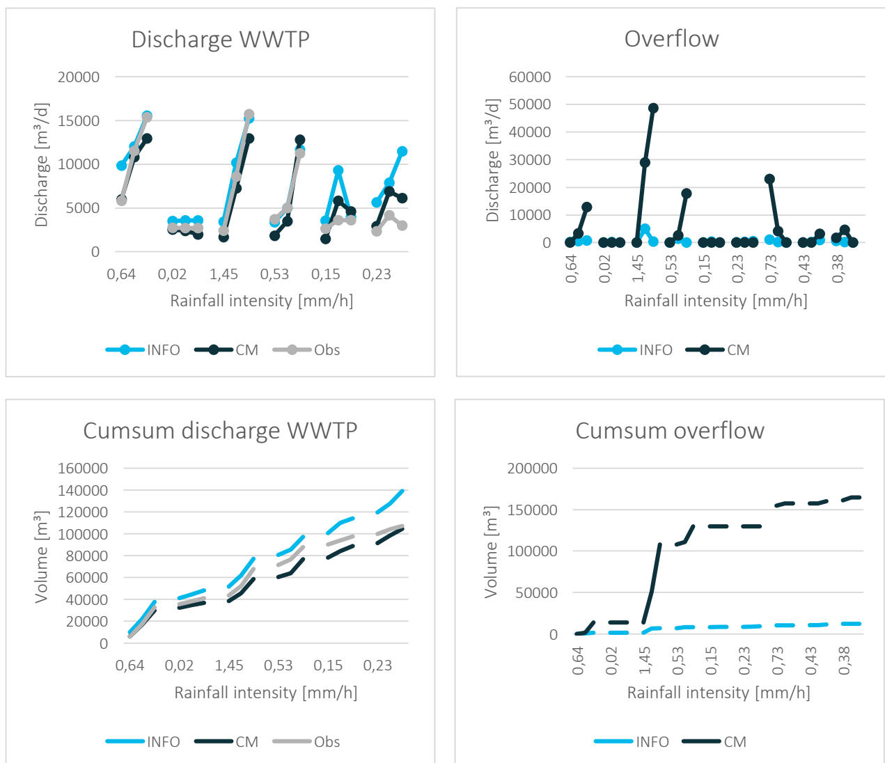
Figure 31: The results from the Infoworks CS model, the CM1b and the observations from the DIVA dataset are compared for the used test events. Left – the discharge at the outlet of the WWTP in Evergem is looked at, as well at the discharges for each event as the cumulative volumes. Right – the overflow volumes are examined. Here also both the time series, and the cumulative volumes are looked at. Since there are no observations of the overflow volumes only the results from the Infoworks CS model and CM1b are examined.
