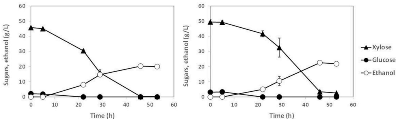
**Fig. 4.** Ethanol production by *S. passalidarum* cultures at 0.2 L scale in bioreactors on medium with (left) a mix of xylose and glucose (reference culture) and (right) on detoxified beech C5 stream (4 g GAC per 100 g stream).
