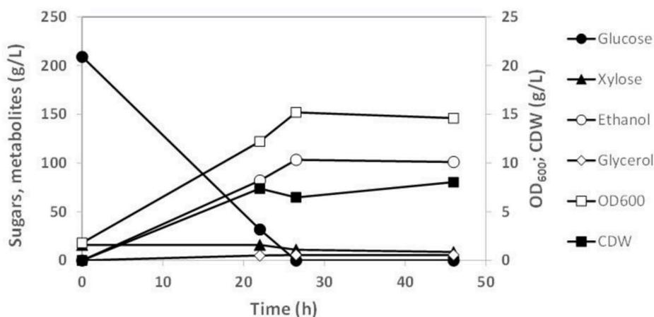
Fig. 5. Fermentation of C6 stream from upscaled fractionation of beech wood chips by *S. cerevisiae* in a 20-L bioreactor with 10 L working volume. The C6 stream was diluted at 50 % (w/v) and supplemented with yeast extract, peptone and salts.
