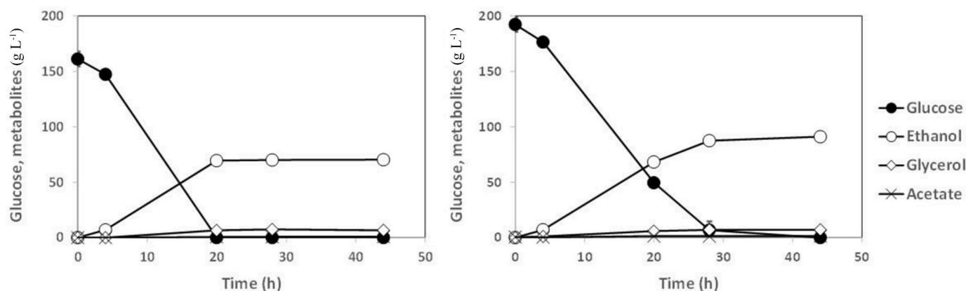
Fig. 2. Ethanol production by *S. cerevisiae* cultures with 0.2-L volume in bioreactors on (right) YP medium with beech C6 sugar stream (C6 + YP) (50 % w/v) and (left) on YPG reference medium.
