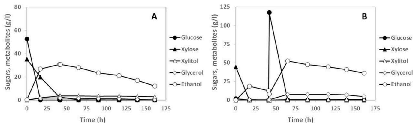
Fig. 8. Substrate consumption and product formation in (A) a co-culture of *S. passalidarum* and *S. cerevisiae* on a mix of pure glucose and xylose; (B) a sequential fermentation of *S. passalidarum* on xylose followed by inoculation with *S. cerevisiae* and addition of glucose at 41 h.
