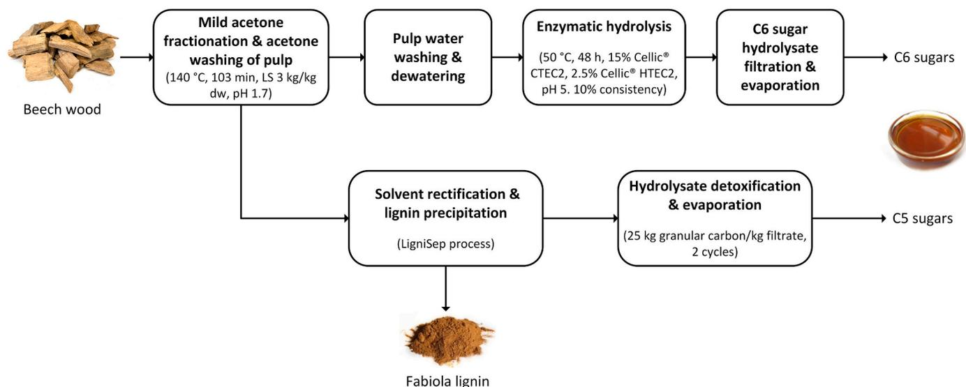
**Fig. 1.** Mild acetone fractionation process, enzymatic hydrolysis and detoxification for the production of lignin, hemicellulose (C5) and cellulose (C6) sugars for fermentation.
