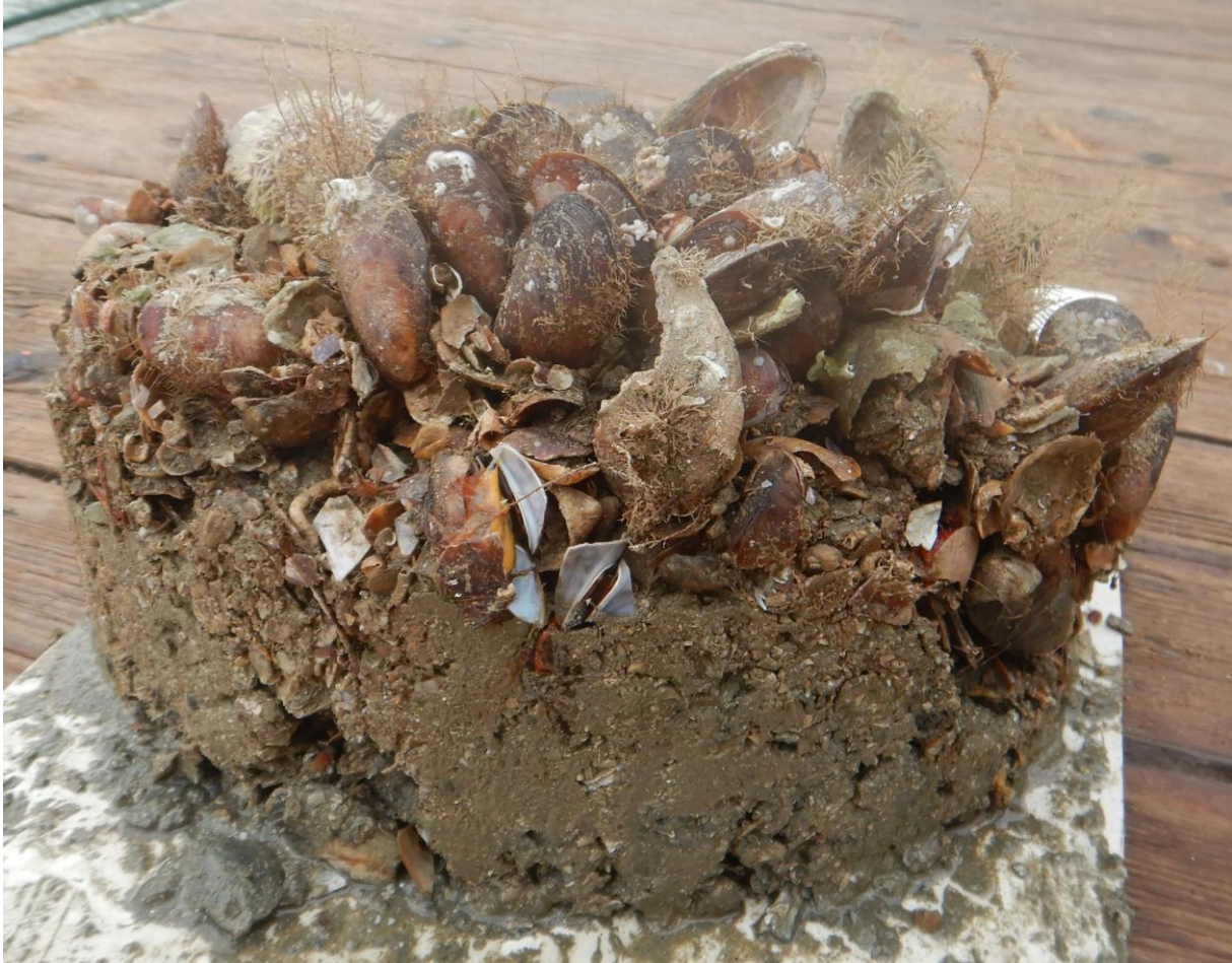
Figure 16: The single core which had penetrated the Modiolus reef and the seabed below it to an acceptable depth. Photo by Rob Witbaard.
