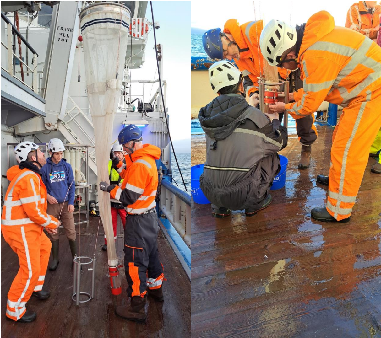
Figure 18: deployment (left) and emptying (right) of the WP2 net. Photos by Francesco Colona
