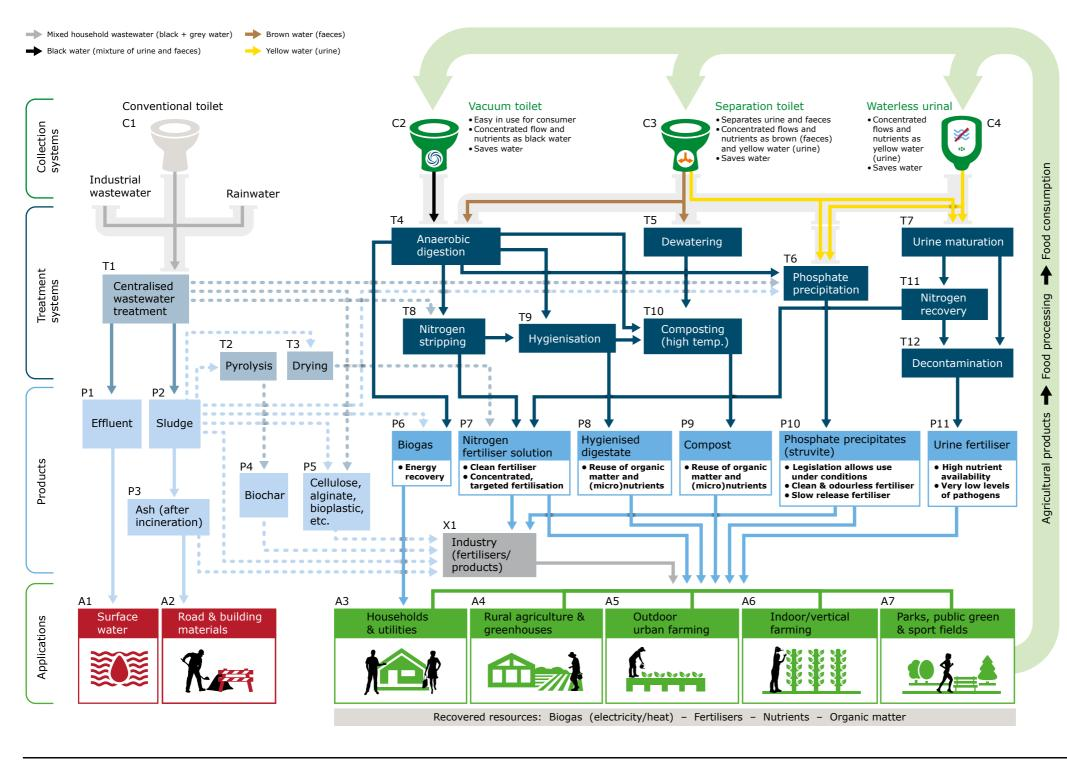
Overview of (present, cetralised) conventional wastewater treatment system (left, lighter colors) and (right, darker colors), and most important/relevant existing and potential routes for recycling of nutrients and other resources (circularity), including collection, treatment, products and applications.
