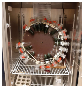
Figure 3. Set-up of batch sorption carousel inside incubator.
