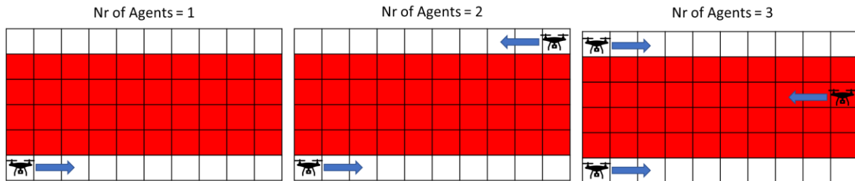
Figure 39: Starting points from agents in LMS . Red cells represent the region where tomatoes were more likely to spawn. The blue arrow indicates the initial movement direction for each agent.
