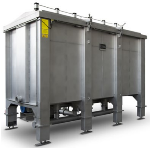
Figure 34 Machine for boiling and bleaching of roving. Photo: Loris Bellini.
