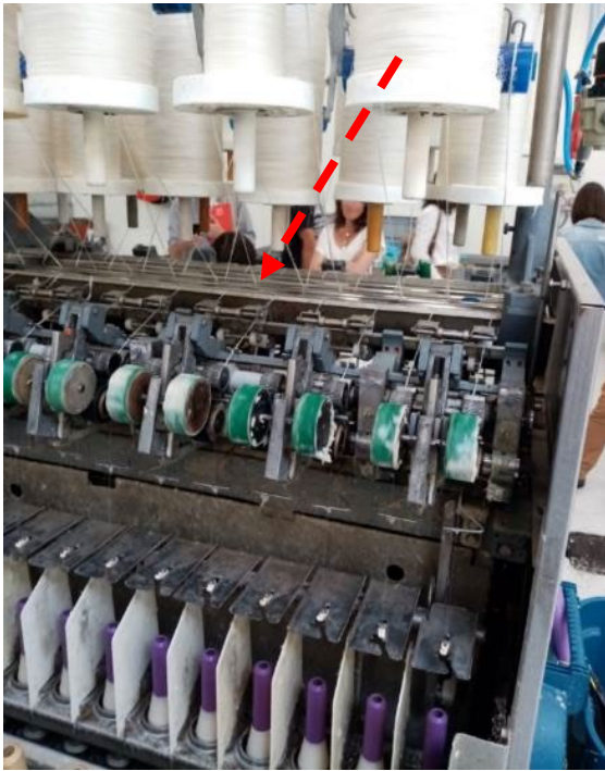
Figure 36 Wet ring spinning of long bleached fibres. The arrow indicates where the yarn passes through the hot water bath. Photo: HOGENT.
