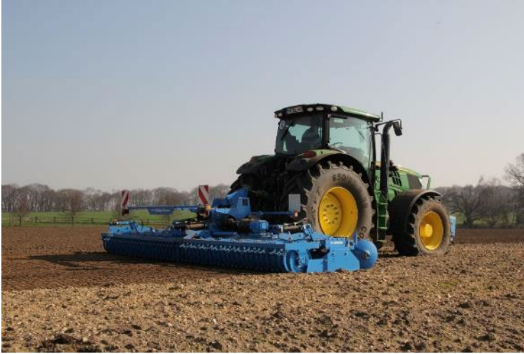
Figure 5 Seedbed preparation with rotor harrow. Photo: HempFlax.
