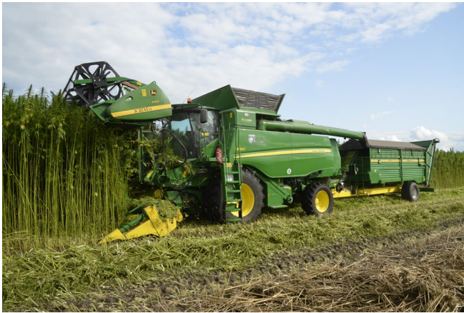
Figure 11 Harvesting machine for fibre hemp, where flowers/leaves are harvested separately. Photo: HempFlax.
