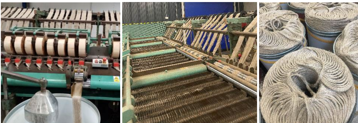
Figure 32 Drafting and doubling of hackled sliver into sliver (left); top view (centre); sliver in barrel (right). Photos: HOGENT.
