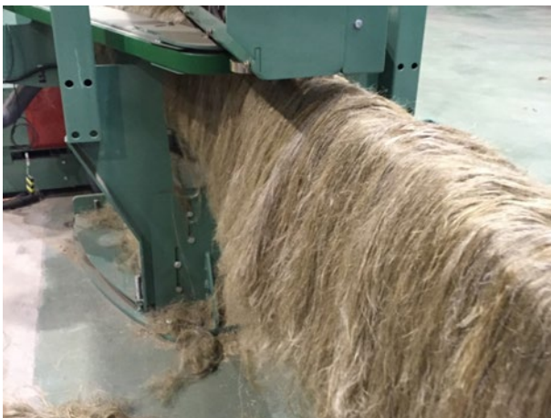
Figure 28 Scutched long fibres leave the scutching line. Photo: HOGENT.
