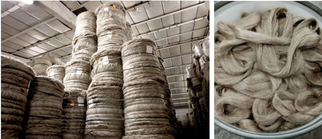
Figure 30 Bales of hackled sliver (left); combed hackled sliver (right). Photos: HOGENT.
