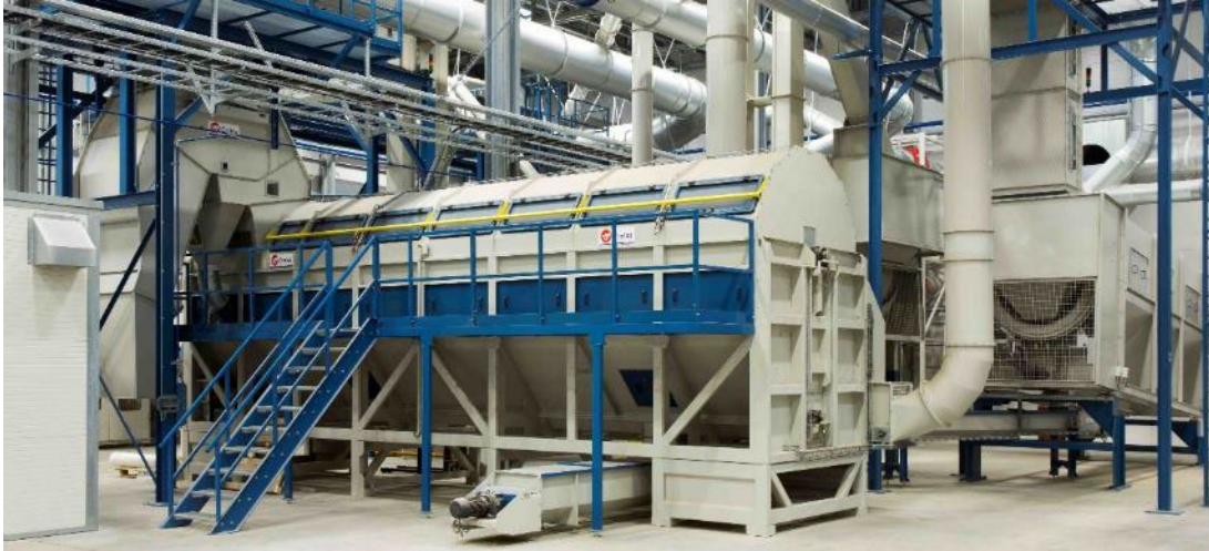
Figure 17 Duvex sieve drum for separating bast fibres and shives. Photo: Cretes.
