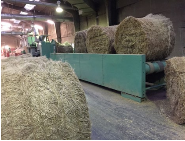
Figure 26 Feeding bales into the scutching line: breaking + scutching. Photo: HOGENT.
