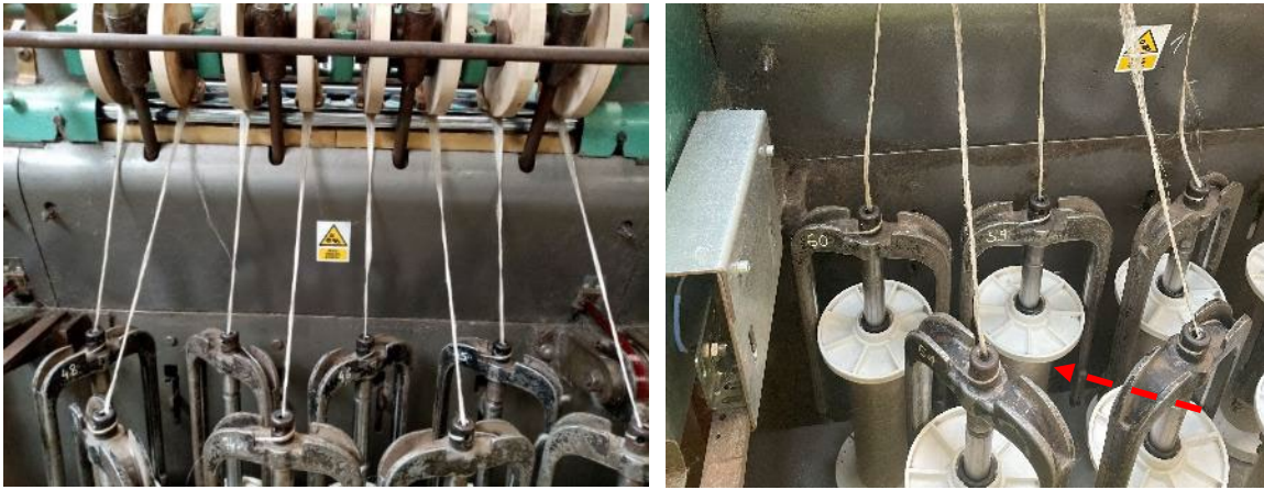
Figure 33 Roving frame for processing sliver into wick on rove bobbin. Photos: HOGENT.
