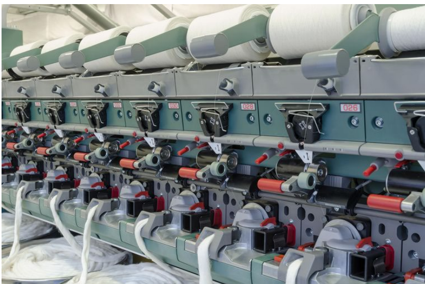
Figure 40 Semi-automatic rotor spinning. Photo: Rieter.
