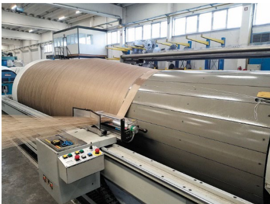
Figure 41 Cone warping machine. Photo: Masureel.
