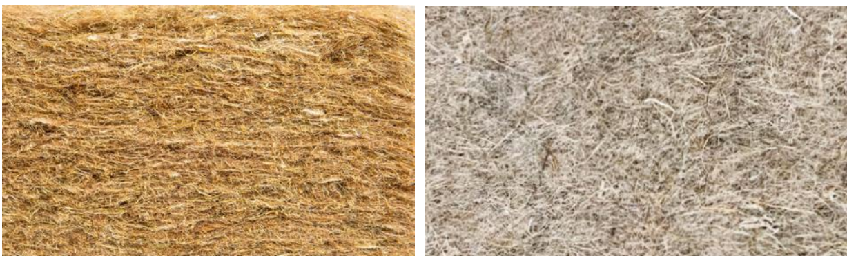
Figure 20 Hemp-based fibre mat for thermal insulation of buildings (left) and for sound insulation, e.g. under floating floors (right). Photos: Thermo-Hanf.
