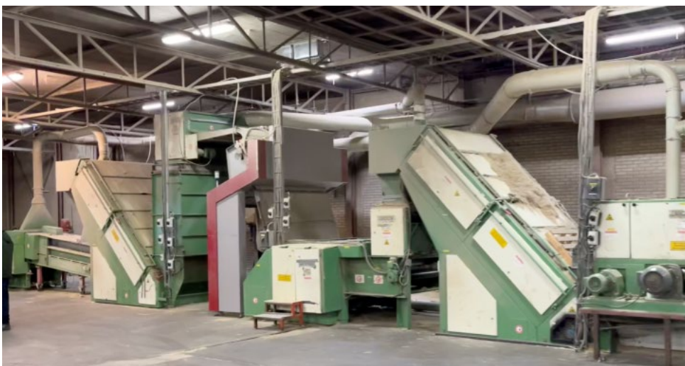
Figure 18 Refining and cleaning hemp fibres. Photo: HempFlax.
