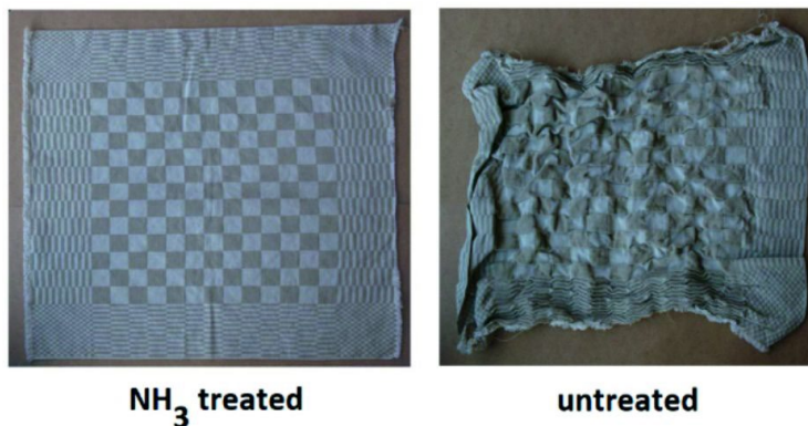
Figure 49 Effect of liquid ammonia treatment on shape stability of hemp tissue. Photo: HOGENT.
