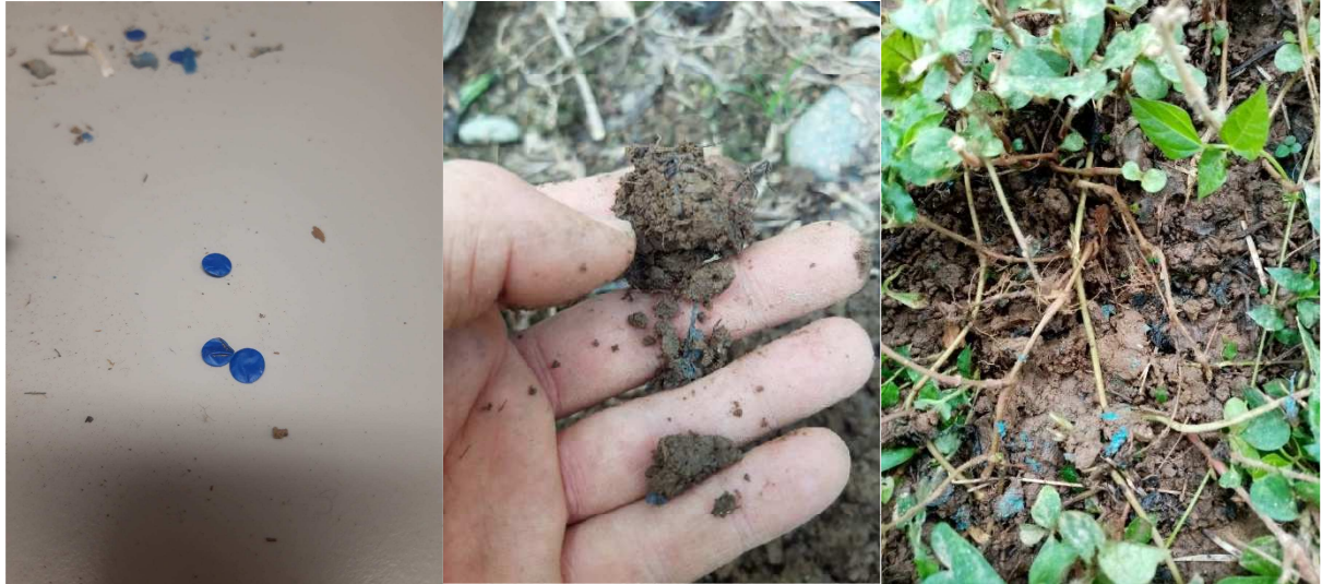
Figure 5: Blue bag macroplastic found in the field: Small disks left after perforation (left), Highly degraded blue bags found within plantation M4 (middle) and V4 (right)
