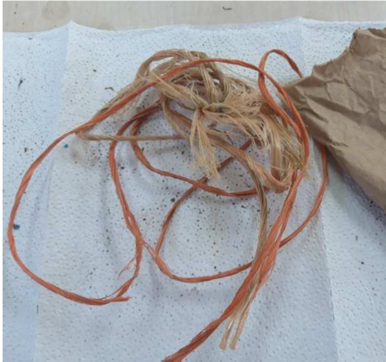
Figure 6: Two strings of twine macroplastic, one very young and the other deteriorated in colour and no longer as tightly woven as the other. Taken from plantation V1 (left),
