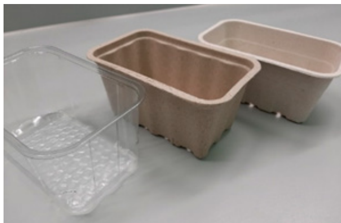
Figure 1 The three types of trays for strawberries that were compared regarding various sustainability aspects (from left to right PET, paddy straw, paper pulp).
