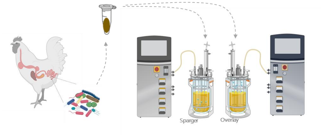
Fig 3. Schematic representation of the gassing strategies testing. The bioreactor on the left shows the nitrogen diffusion into the media, while the one in the right shows the nitrogen overhead flushing.
