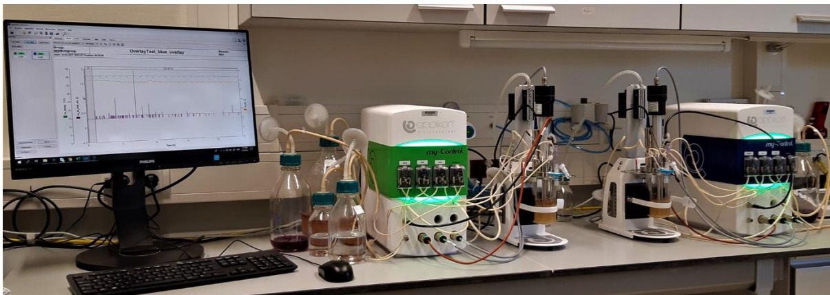
Figure 5. Set up of in vitro chicken caecal system. The system includes two 250 ml bioreactors (control and treatment) operated in parallel with a semi-automated workflow with all the parameters needed to simulate some physiological conditions of the chicken caeca. Target parameters are controlled by two computers and dedicated software.
