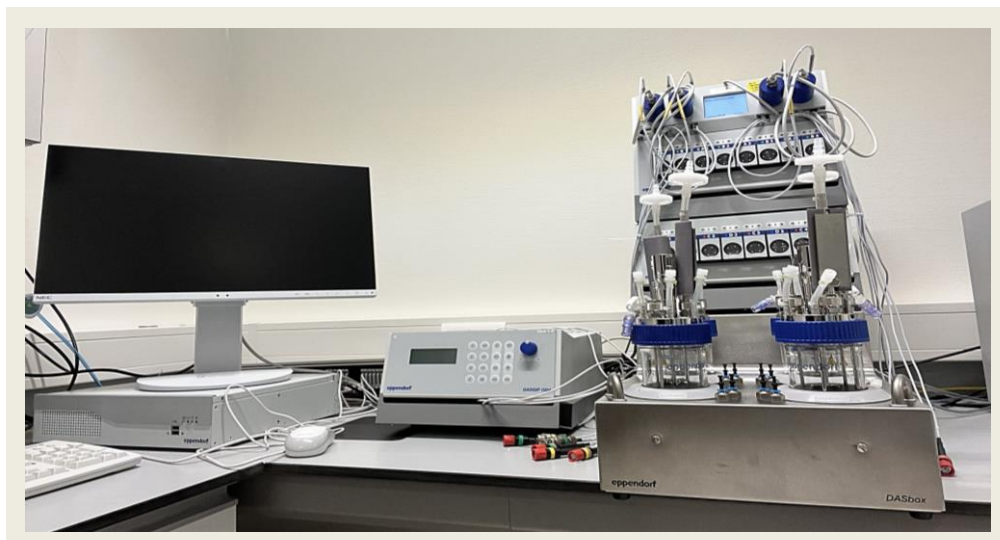
Figure 8. DASbox system. Four-fold system supporting working volumes of 60 to 250 ml and real time monitoring of the critical experimental conditions.
