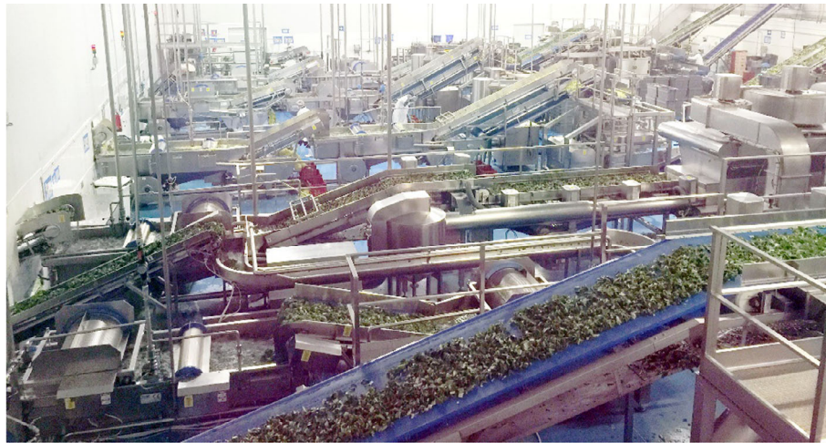
Figure 4: Fresh-cut processing plant including the washing tanks and the flumes. © A. Allende
