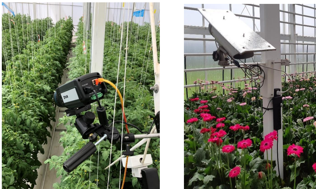
Figure 28 Imaging thermal camera. On the left when used in a short-term measurement, on the right built into a housing that protects the camera from overheating by the sun. In this project, the set-up shown in the right image has always been mounted above the 4 crops during a number of summer days.
