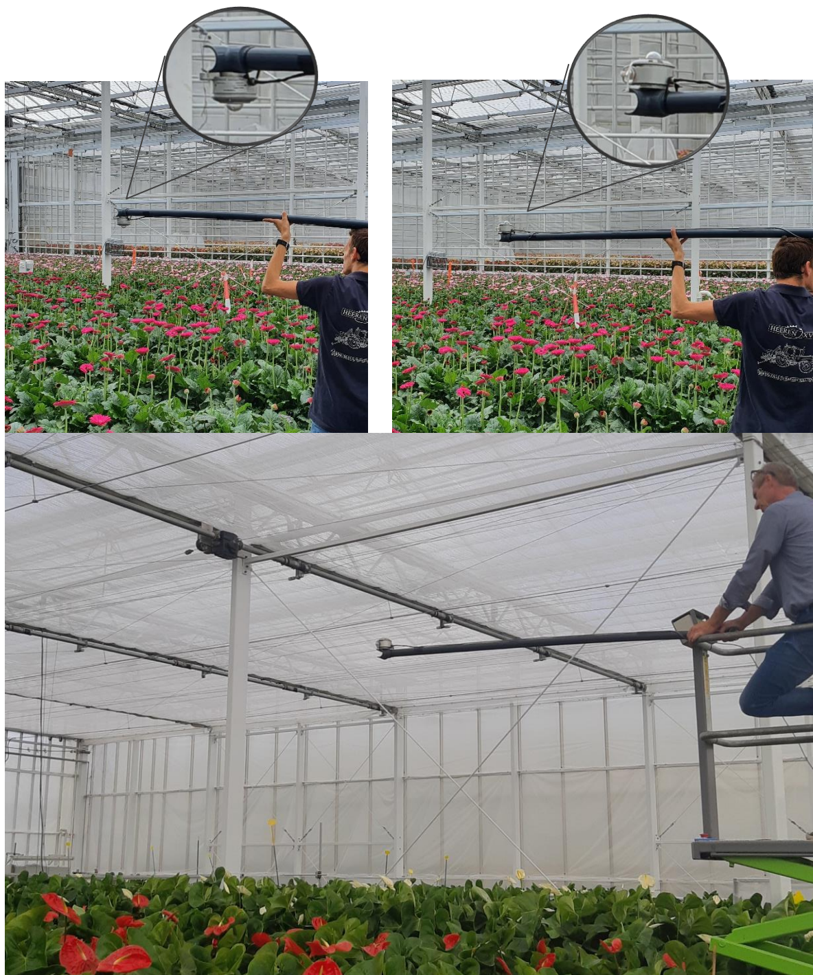
Figure 12 Manual determination of light absorption by crop+floor by measuring the downward and upward short-wave radiation.
