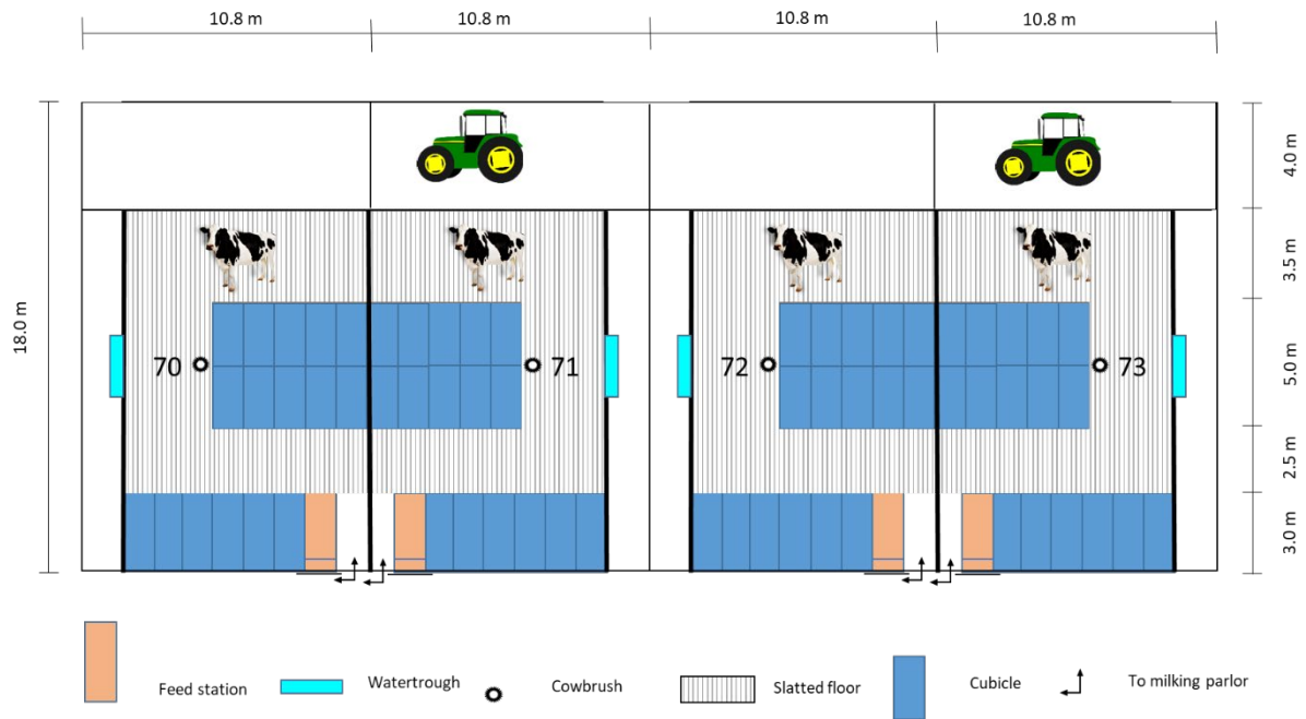
Figure 3 Detailed lay-out of the four cubicle rooms. The CowToilet was installed in unit 70 (case) and unit 72 served as the control.
