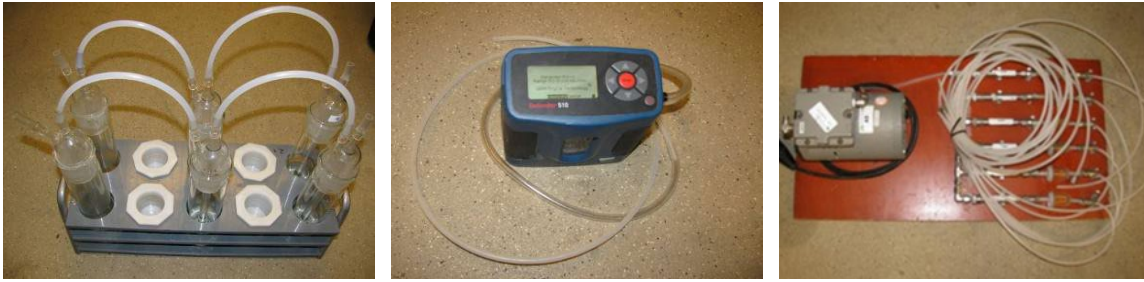
Figure 8 Set-up WLR gas washing method. Left: absorption flasks (measurements in duplicate; per train (in series) two absorption flasks filled with absorption medium and one empty absorption flask for protection of the pump). Middle: Dry gas flow meter (DryCal® Defender 510-m, Bios Int. Corp, USA). Right: pump (Thomas Industries Inc., model 617CD32, Wabasha, Minnesota ,VS), sampling lines (Teflon or polyethylene), and critical orifices (borosilicate glass (diameter: 8 mm; length: 80 mm), housed in a stainless steel container for protection; flow: ~1000 ml/min).
