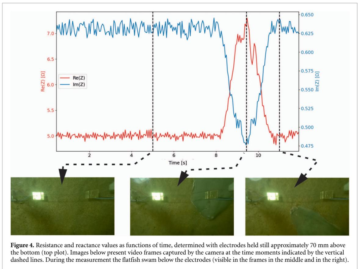
The described results were obtained using electrodes dragged approximately 70 mm above the bottom. Such a close-range detection setup should be suitable for bottom fishing, in which sensors integrated with the fishing gear are dragged just above or directly on the seafloor (Boute 2022). The exact relation between the achievable detection performance and distance from a fish is complex, depending on
