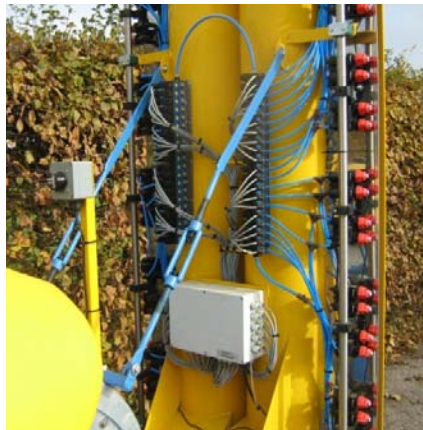
Fig. 1. The Canopy Density Spraying system is equipped with a Hokuyo URG-04LX laser scanner and with Lechler VariosSelect pneumatic actuated nozzle bodies. The sprayer used is a KWH D-1000 orchard sprayer and the nozzles are clustered in groups of four.
