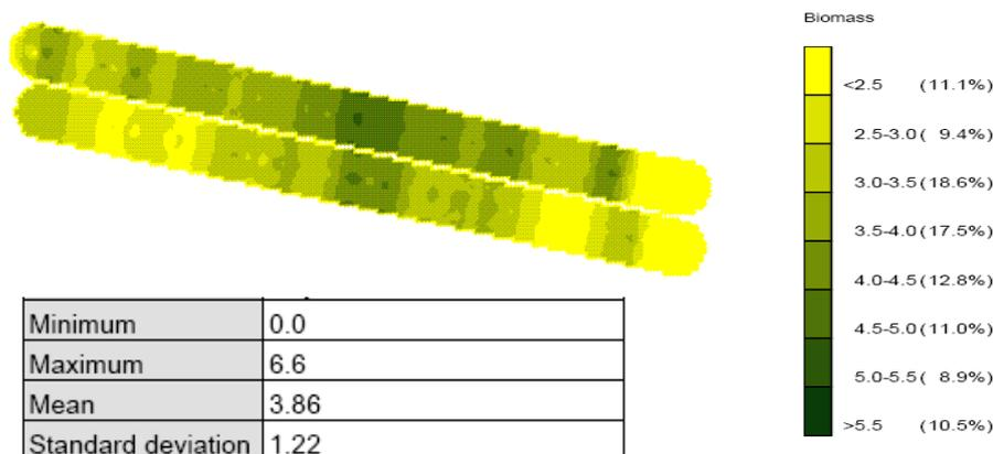
Fig. 1. Biomass map (top left) of two bands in a ware potato field made with Yara ALS N-Sensor (Biddinghuizen, 2008). The legend relates colours to biomass-parameter ( $S_N$  value). The Table contains minimum, maximum, mean and stdev of  $S_N$ .
