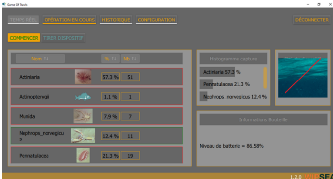
A user interface displays the catch information (species and relative composition) and device status to the skipper in real time.
