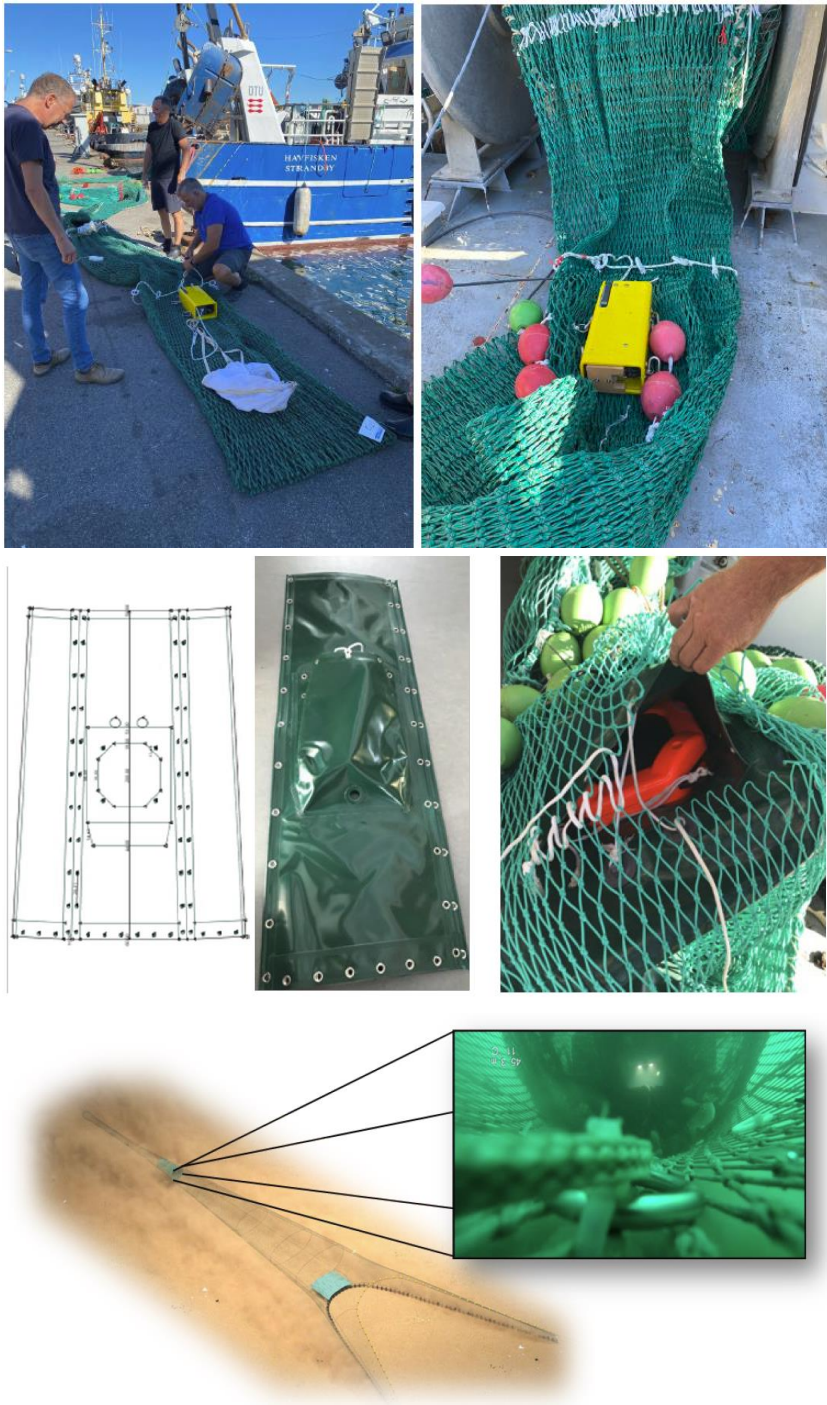
Design of the observation scene with easy-access TrawlMonitor integration in a pocket. System integration in a Norway lobster trawl and system in operation during demersal trawling. Source: modified and adapted from Krag et al. (2022).
