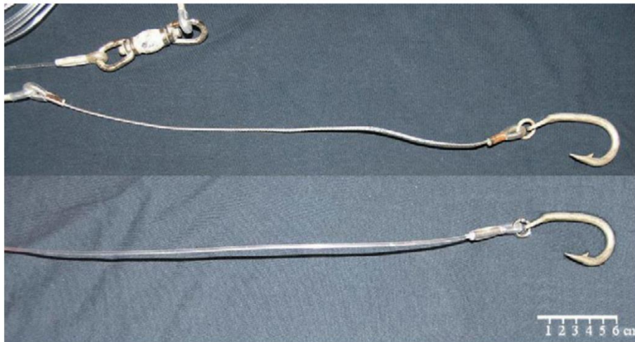
Wire leader (top) and nylon leader (bottom). Only the type of leader differs. Source: modified and adapted from Ward et al. (2008).
